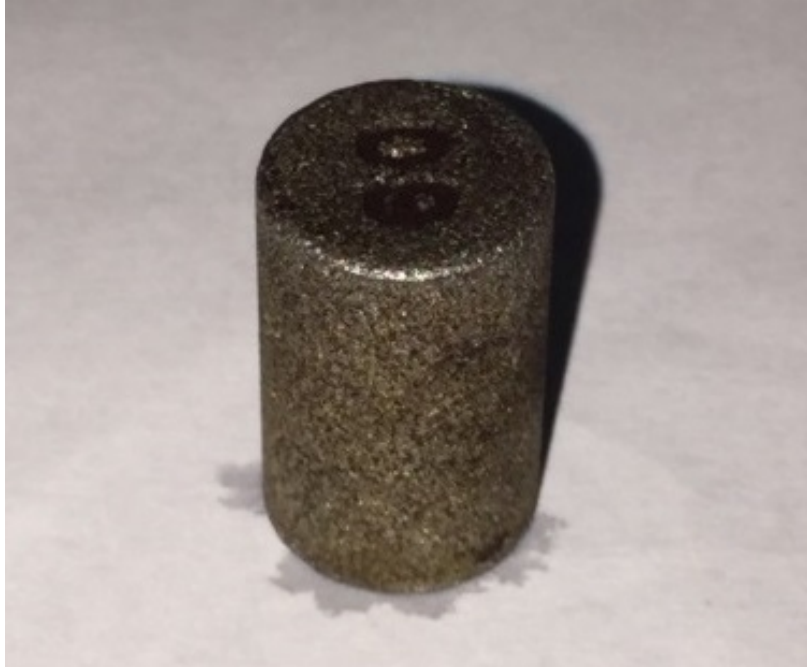
Figure 3: Example of Plugged Inline Sample Filter
