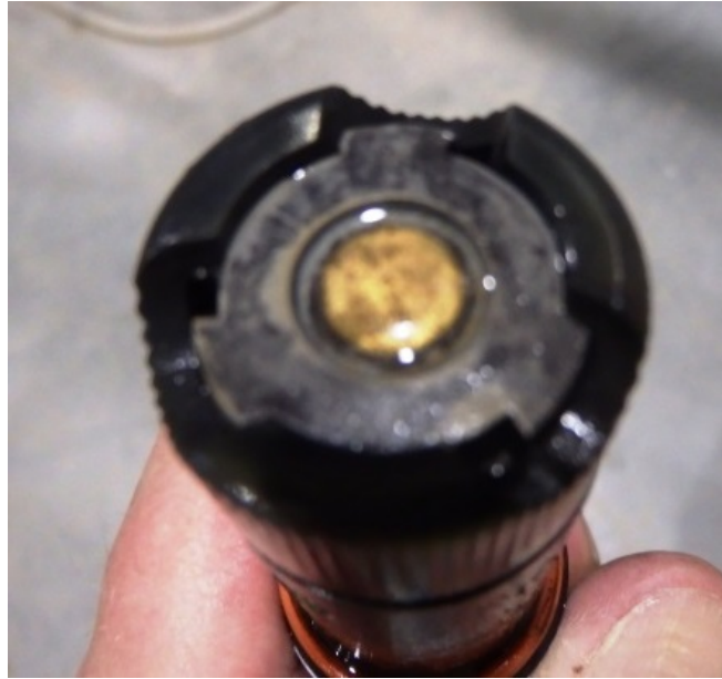
Figure 5: Example of Fouled Dissolved Oxygen Probe
