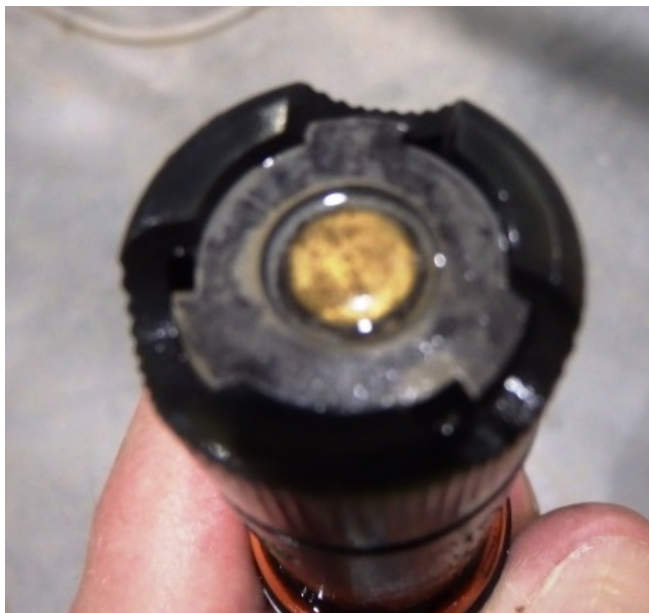
Figure 5: Example of Fouled Dissolved Oxygen Probe
